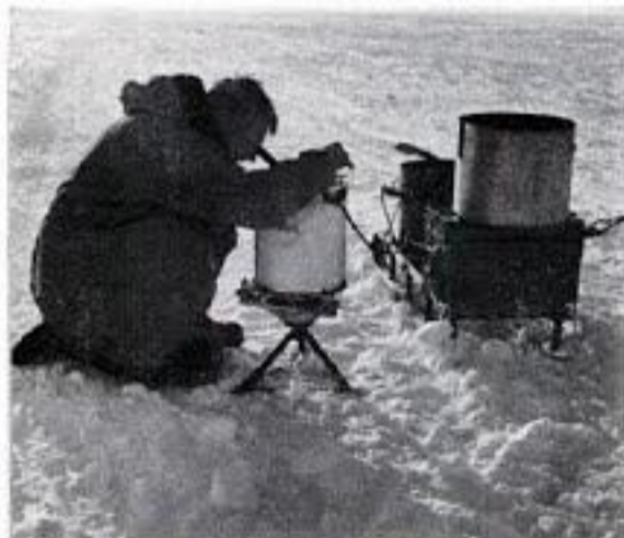
MEASURING GRAVITY , Scientist Robert Cottell determines earth's gravitational pull. Force of gravity is stronger near the Pole than it is at equator.
